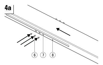
Applies only to: KOOI-REACHFORKS® type TRG2; Slide the (new) inner sleeve (8) onto the fork. Tighten the screws (6) (on both sides in the stops (7). Lock the screws (6) with Loctite 270<sup>1</sup>.
