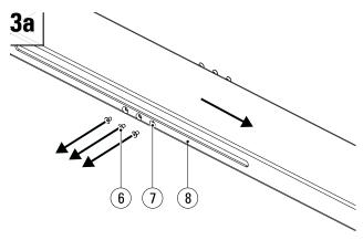
Applies only to: KOOI-REACHFORKS® type TRG2; Unscrew the screws (6) (on both sides) from the stops (7) and remove the inner sleeve. **Tools required:** Allen key 4.
