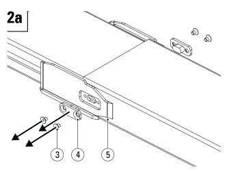
Applies only to: KOOI-REACHFORKS® type TRG2; Unscrew the screws (3) and remove the stops (4) from the outer sleeve (5) (on both sides of the sleeve). **Tools required:** Allen key 4.
