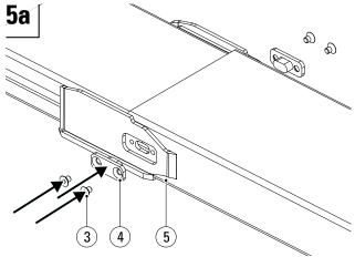
Applies only to: KOOI-REACHFORKS® type TRG2; Place the stops (4) in the outer sleeve (5). Tighten the screws (3) (on both sides od the sleeve). Lock the screws (3) with Loctite 270<sup>1</sup>.
