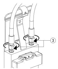
Screw the hose connectors (3) tight. **Tools required**: Open-ended spanner 22.
