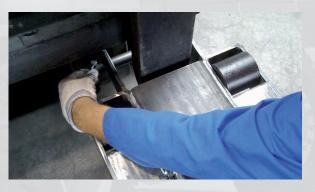
**Rollerized Tine Extensions** are very easy to fit onto the existing lifttruck forks just by using a locking pin.
