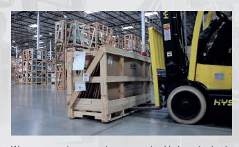
Wrong procedure as the mast should be absolutely vertical. Take control of these problems, by using the KOOI-FLATFORKS Indicator®
