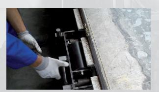
**Rollerized Tines** come standard with stop-mechanism to prevent cargo pallets from rolling off the tines.
