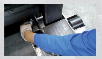
Rollerized Tine Extensions are very easy to fit onto the existing lifttruck forks just by using a locking pin.
