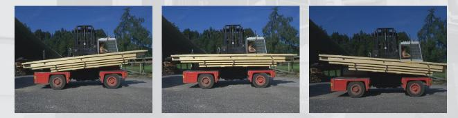
When used in combination with KOOI-REACHFORKS® (hydraulic extendable forks) the Single Height Shift System (SHSSL) can be operated for one sided loading and unloading but also one of the hydraulic forks can operate independently. Which makes the forklift truck much more flexible.
