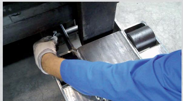
**Rollerized Tine Extensions** are very easy to fit onto the existing liftruck forks just by using a locking pin.
