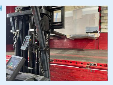
With the KOOI® Control system, operators can now precisely set the desired fork length. The system allows for either visual stopping or fully automatic extension control. In automatic mode, multiple presets can be configured. When a preset length is reached, the oil flow is temporarily cut off, pausing fork extension. After a few seconds, the system reactivates, allowing further operation if needed.
