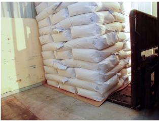
Once the load is positioned on the Roller-Forks, it can be transported into the container or truck. When the RollerForks make contact with the floor, the rollers will move upwards, and as the forklift reverses, the load will remain in the same position. This is due to the RollerForks' principle of a double-layer roller system, where the rollers always rotate in opposite directions.
