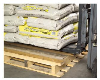
Convert a standard pallet into a "RollerForks Pallet" to quickly and safely remove the load from the pallet without causing damage. The additional inserts, created by placing extra beams on the top deck, allow the RollerForks to easily maneuver under the slipsheet, making it simple to position loads like bagged goods onto the RollerForks.
